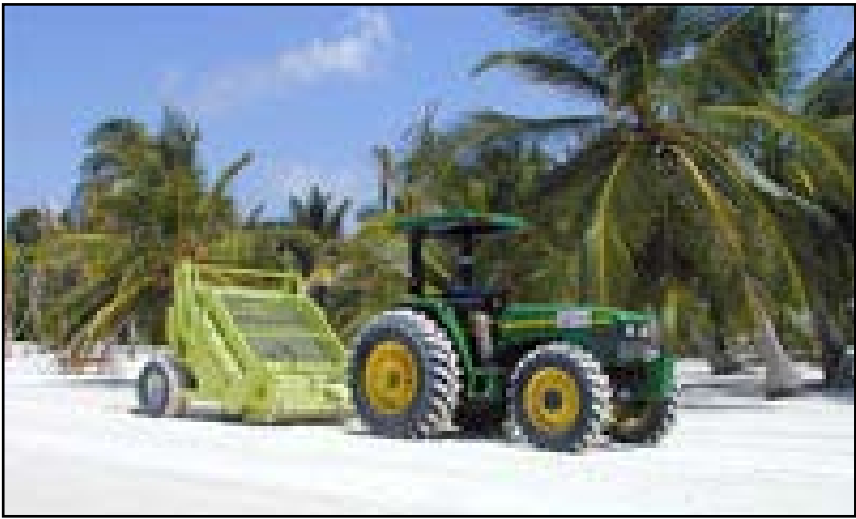
TRACTOR TOWED BEACH CLEANER Image: M. Barber & Sons
